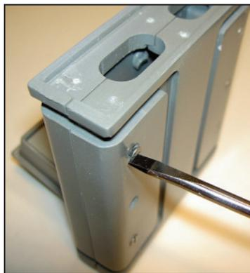
**Step 12:** Put the brass axle through the holes in the fold-out door and slide it into place, and screw the 2 halves of the base together with the long wood screws. You can use some CA glue to help hold them together if you wish, keeping in mind that if you're going to install electronics later you might not be able to get glued parts apart without causing damage.
