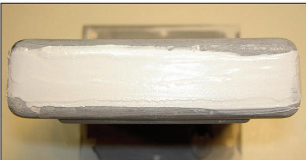
**Step 16:** Bondo or putty the seams down the visible sides of the lower body that the rubber grips won't be covering, and the bottom, as well as the seam at the middle sides of the top wedge/mid-plate, and sand with 400-grit paper until smooth.
