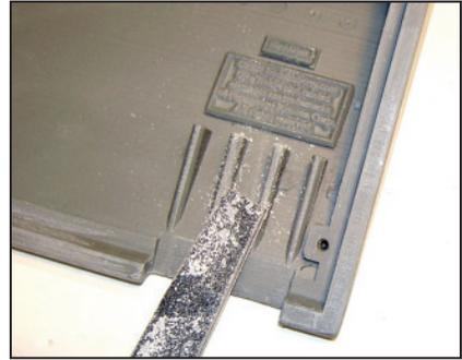
**Step 14:** Sand and assemble the data chip slider by gluing with Weld-On 3 the cross shaped piece (the long side) to the oval thumb-slider through the hole on the mid-plate with the cross piece towards the inside, making sure it will still slide easily -- you should also sand smooth the areas on the mid-plate and the top wedge where the slider and data chip will be in contact for smooth operation.
