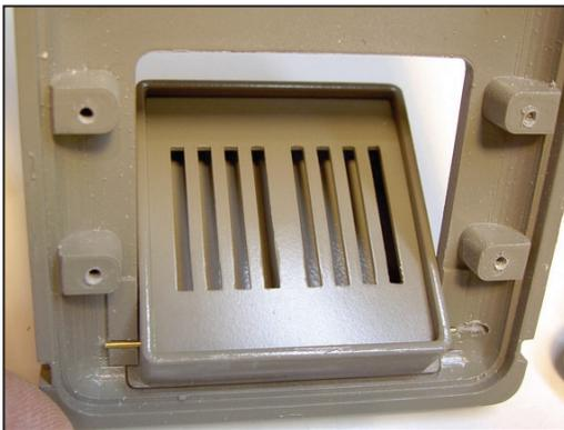
**Step 11:** Glue the top 8 slot chip-holder plate, which is placed paint side out on top of the spacer piece and on the back two resin axle areas.
