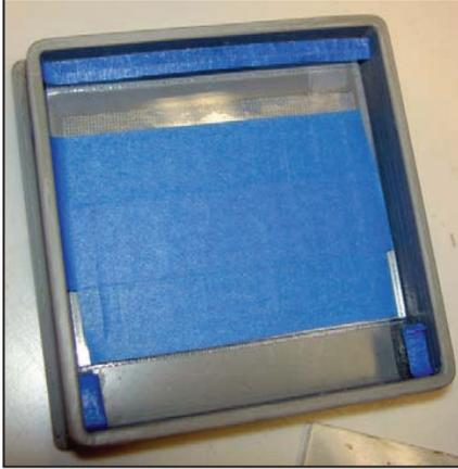
**Step 10:** With masking tape, mask the lower slot plate covering all the slots, and the top surfaces of the two axle protrusions and the spacer plate .
