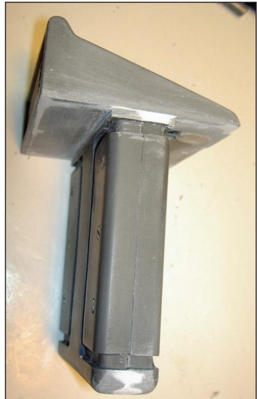
**Step 18:** Make sure to close the chip door to ensure no additional paint gets inside, and spray primer all of your tricorder. Check the surface for imperfections, putty and sand any such areas, and primer again until you are satisfied with your finish. Paint with Krylon Stone Gray, wet sand if desired with 600 grit, then paint a final coat of gray and set aside to cure several hours or overnight. A gloss finish is best for application of water-slide decals.
