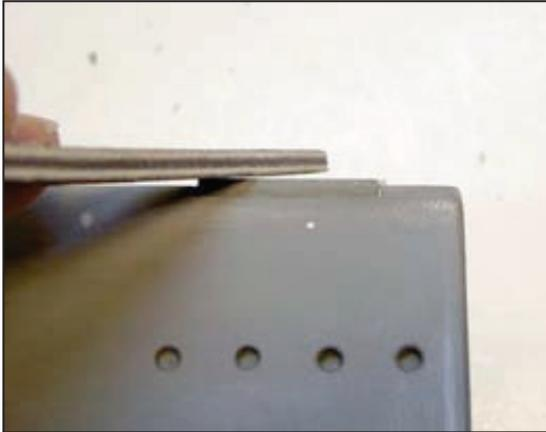
**Step 17:** File or sand the chip slot lip until it is even with the tricorder's edge if needed.
