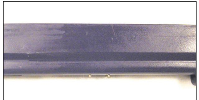
**Step 6:** Once in place, be certain that all the pins are straight and stick out exactly 1/16". Then **CAREFULLY** spot glue them into place by applying a small amount of CA glue to each one on the inside of the compartment. **Be careful not to get any glue on the front of the pins!!**
