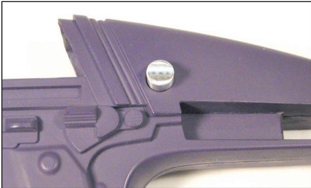
**Step 14:** Next, permanently attach the completed switch/knob assembly to the inside of the phaser body, following the instructions listed in the prop kit instruction manual. Test the action of the switch to verify smooth operation.
