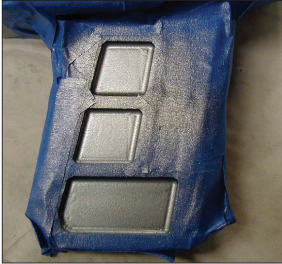
Masking and final paint finish of handgrip.
