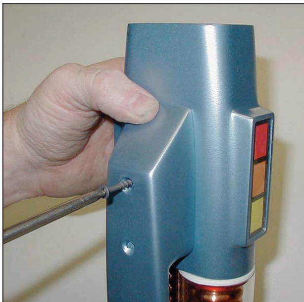
Drilling and screwing on the rear body to the rifle.
