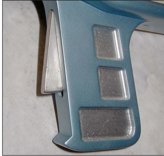
Masking and final paint finish of handgrip.
