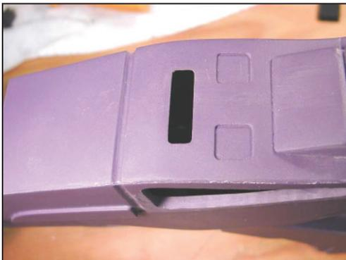
**Step 3:** This photo shows the cut out for the LED power graph. Precise size and shape are critical here, and careful use of a dremel tool and various files are recommended to make this hole.
