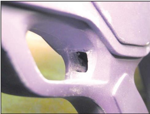
**Step 6:** This photo shows a small square hole for the trigger switch cut out of the trigger location above the handle. The hole is approximately  $1/2$ " in diameter.
