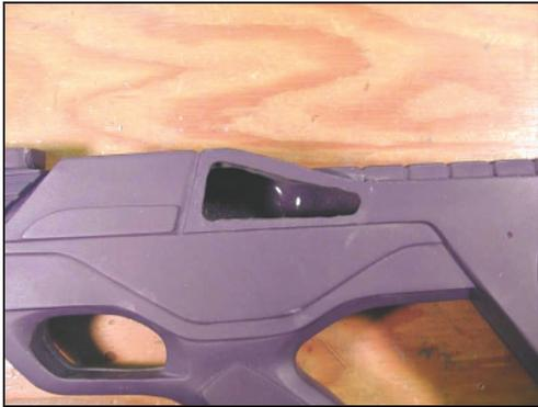
**Step 1:** This photo shows the access hole cut out of the rear left side of the rifle panel. Carefully use a dremel tool to accomplish this step. This hole is for the power graph LED circuit installation and battery storage.
