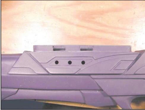
**Step 5:** This photo shows the (2) rectangular holes for the power switches cut out of the side of the scope riser. The holes are approximately  $11/16$ " X  $1/4$ ".
