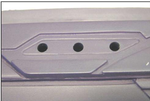
**Step 2:** This photo shows the (3) holes drilled out on the mid left side panel under the scope for the 3 LED trio.
