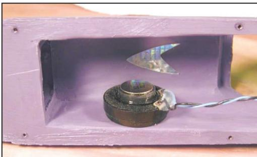
**Step 10:** For optimum sound volume, the speaker should be mounted face down against the inside of the scope wall using hot glue.
