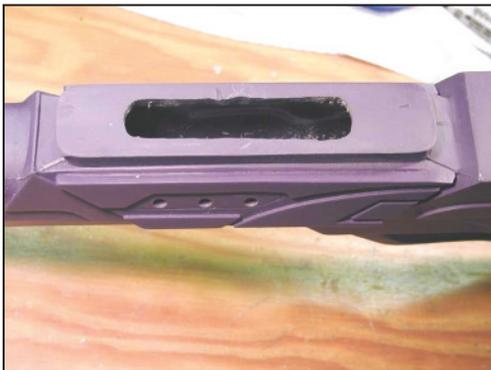
**Step 4:** This photo shows a 3” slot cut out of the riser, where the scope will be attached. This is for the installation of the 3 red side light LEDs, as well as the storage/housing for the main circuit board and sound/emitter module. It also serves as a “connection point” for the wires coming from various locations in the rifle, addressed later in these instructions.
