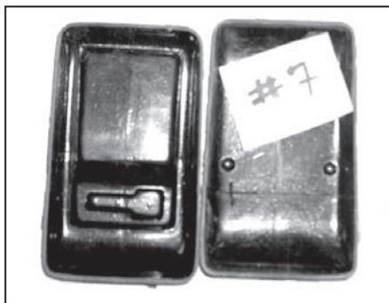
**Step 3:** Flat sand (with 180 - 220 grit) the flat edges of the upper and lower black body shells just enough to get rid of the die cuts, and to even the edges. **Don't press too hard. Let the sandpaper do the work.**
