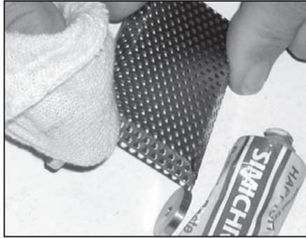
**Step 1:** The brass grid can be polished with a brass-polishing compound. You can spray a lacquer coating over the polished and cleaned grid, if you desire to. But leaving off the lacquer is recommended, so you can clean and re-polish when the grid gets dull or oxidizes.
