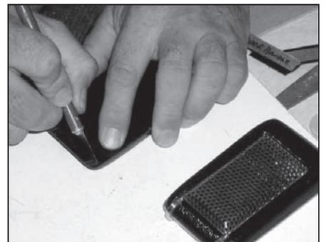
**Step 15:** Lay the back shell onto the bottom of the mid-plate. Line up the back with the grid wheels, and mark on the back shell in the same way as you did with the top shell. Cut squarely down to the line marked inside. Cut the excess plastic strip out.
