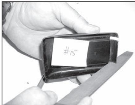
**Step 5:** Mark on the upper shell where each side of the wheels sits as close as possible. Squarely make the 2 cuts down to the top of the inside lip. Cut across the 2 cuts in each slot and remove the plastic strip. Test fit the grid to make sure it fits all the way to the front end of the shell. File the slots where the wheels fit in. *Do not over cut or over file the slots. You want the slots to be just big enough to fit the wheels.*
