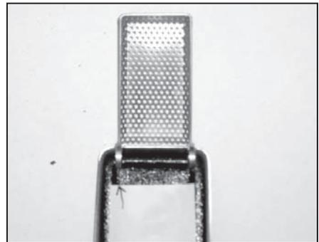
**Step 7:** Place the top shell on the mid-plate, and check the fit to see if the grid closes easily. If too tight, file a little more towards the inside of the body to make room to slide the grid inwards. Look to see if the top shell is fitting the mid-plate evenly. There should be a small amount of the metal edge showing evenly around the top shell. Make sure you have cut away just enough plastic to fit tightly to the wheels, but still have free movement.
