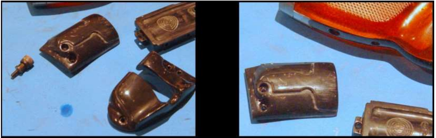
Pictures 05 & 06: The metal side covers and the magazine were sprayed black and then careful attention was given to creating the scuff marks that are seen on the original
