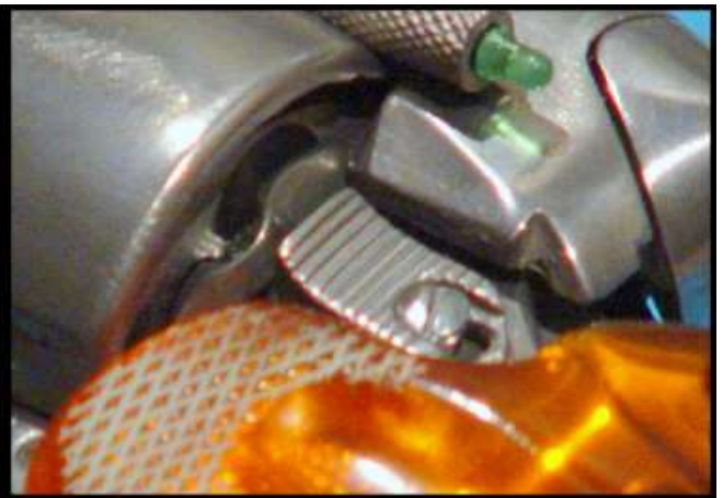
Picture 03: Filing and setting the fit of the Steyr bolt assembly / Picture 04: The Bulldog release catch screw was totally incorrect - it required extensive remodeling and polishing
