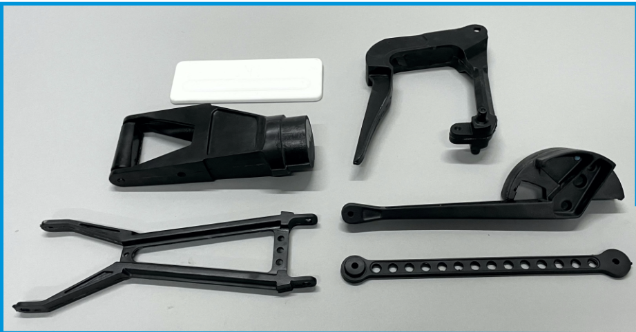
Landing Gear locks. 6 pieces cast urethane, 1 vacuum-formed part,
