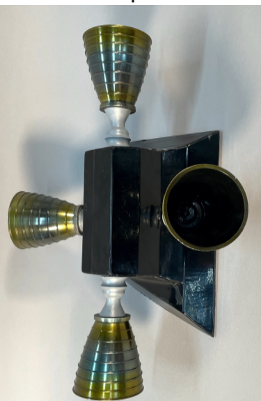
RCS thruster Quad 4 sets per LM
