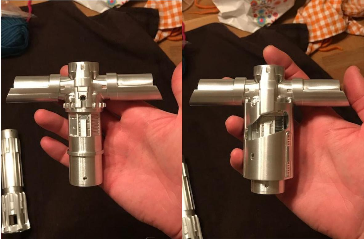
When you want to add in the red wire, look under the saber with the core out. There is a 3mm hole to the left of the spacer location, under the saber. The wire will simply be plugged in and the wire will stay in place without any glue.
