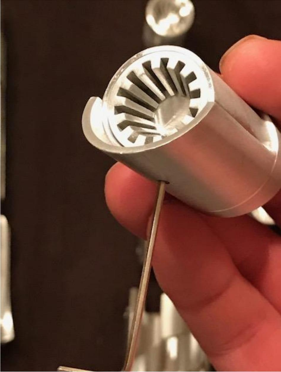
To remove the mainblade/core there are 2 M3 set screws under the shroud on the back side.
