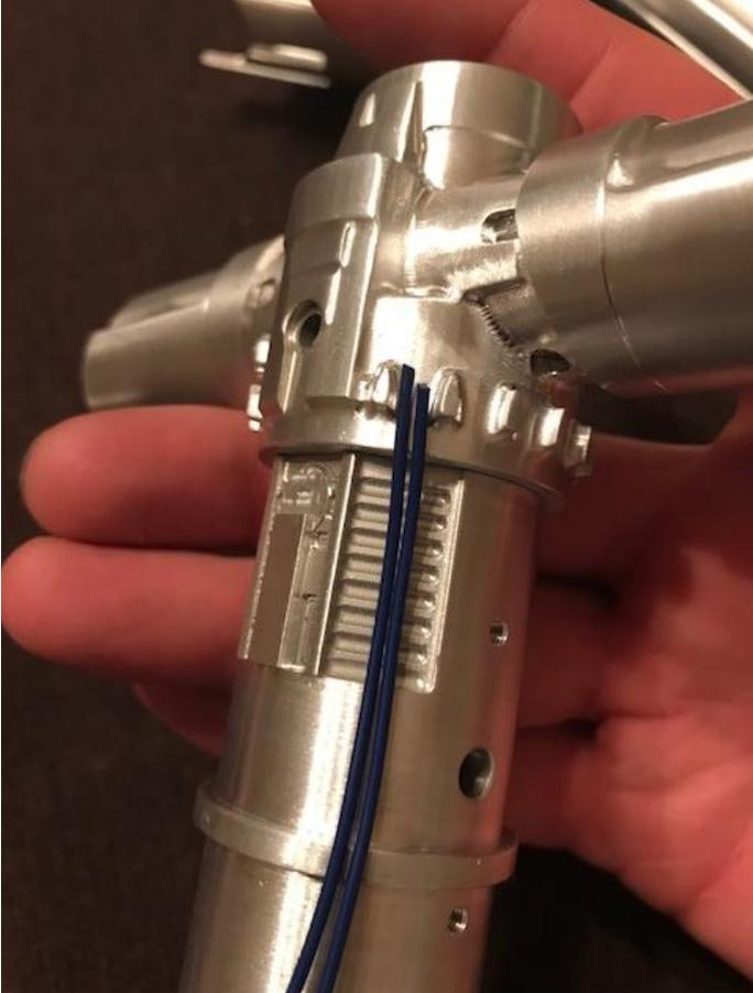
You can see one of the round head screws that holds the shroud, lower and upper section all in place. There are 2 more to the left and right of this along the side. These screws are M3 and please be careful when tightening these to prevent stripping. Tighten them down but don't go all Hercules on them. It's unnecessary.
